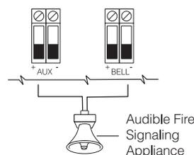
For UL installations, when a bell or siren is used for fire signaling with a pulsed cadence, it must be connected between the AUX+ and BELL- terminals. To maintain bell circuit supervision, do not connect more than one device to the BELL-terminal. A fire bell or siren
