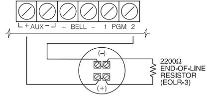
**NOTE:** If PGM2 is programmed for 2-wire smoke support, Jumper CON1 on the main board must be removed.
