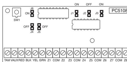
**NOTE:** Only jumpers J1, J2, and J3 determine the zone assignment for the module.
