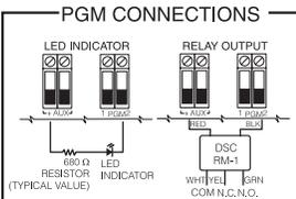
**IMPORTANT:** Minimum 6.4mm (0.25 in) separation must be maintained between RM-1 circuits and all other wiring.
