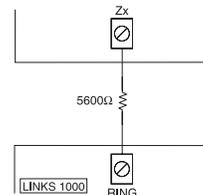
If the LINKS1000 cellular communicator is being used a zone may be configured for LINKS1000 Answer to allow downloading to be performed in the event of telephone line failure. When the LINKS1000 receives a telephone call it will activate the RING terminal on the LINKS1000 circuit board.
