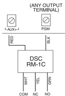
Each PGM output is designed so that when activated by the panel, the terminal will switch to ground. PGM1 can sink up to 50 mA of current. These PGMs can be used to activate LEDs or a small buzzer. Connect the positive side of the LED or buzzer to AUX+, the negative side to the PGM.
